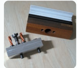
DRILLING OF WOOD AND PVC WINDOW FRAME TO FIT CREMONE BOLT Page 16.11
