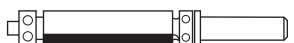
HW FLUSH TRIM BITS WITH UPPER AND LOWER BALL BEARING Z=2 Page 2.16
