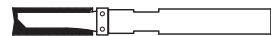
HW "MINI" FLUSH TRIM BITS WITH UPPER BALL BEARING GUIDE Z=2 Page 1.21
